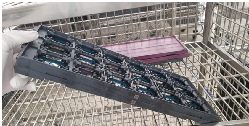
Figure 5: LCP Tray stability during tilt-and-shake DOE.
