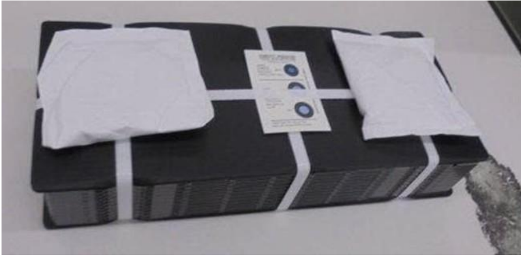
Figure 4: TFT tray stack prepared and tightened before vacuum sealing
