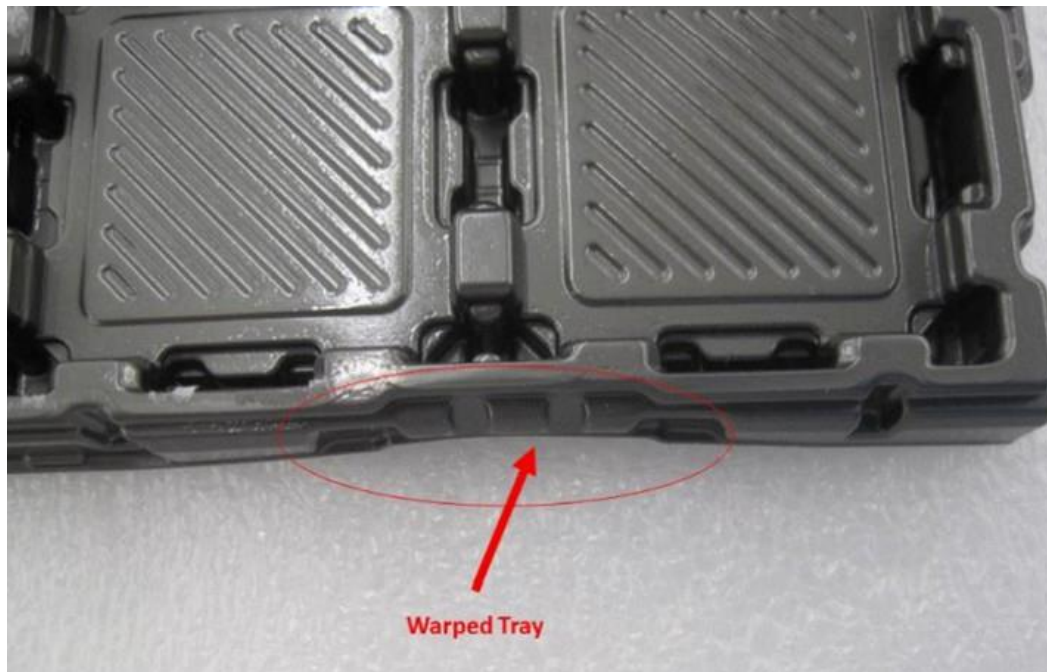
Figure 3: TFT deformation after BNS sealing, resulting in non-reusable trays
